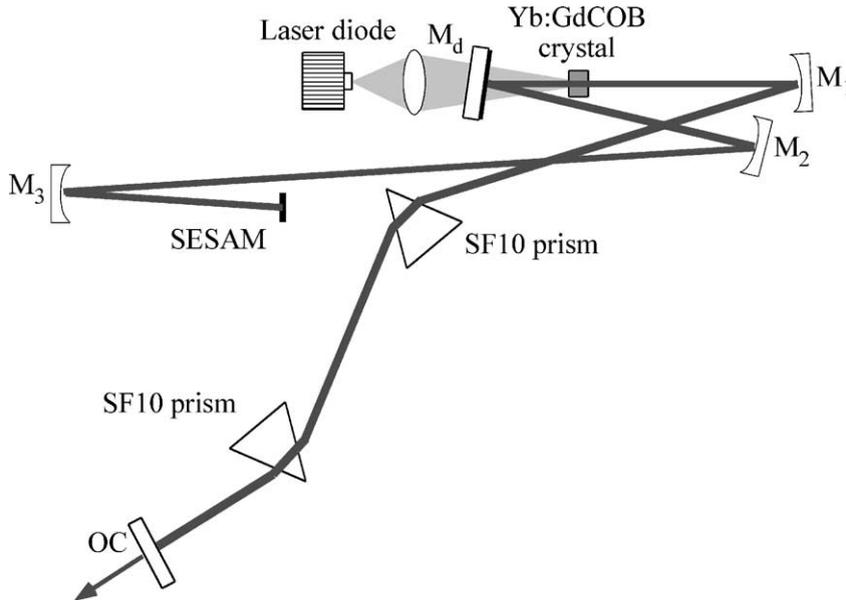
Fig. 8. Experimental setup.  $M_d$ : dichroic mirror;  $M_1$ ,  $M_2$ ,  $M_3$ : HR mirrors with, respectively, 30-mm, 20-mm, and 15-mm radius of curvature; OC: 1% or 2% transmission plane output coupler; SESAM: high-finesse SESAM.
