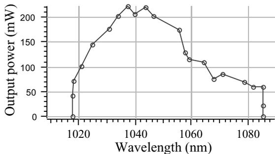
Fig. 4. Tunability of the CW Yb:GdCOB laser diode pumped at 976 nm.
