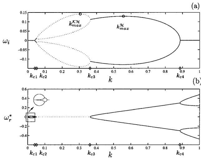
FIG. 3. (a) Temporal growth rate  $\omega_i$  and (b) intrinsic frequency  $\omega_r^* = \omega_r - ak$  with respect to the real wave number  $k$  for  $R_i = 0.04$ . The dotted curve shows the Kelvin–Helmholtz modes.
