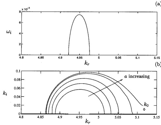
FIG. 11. Comparison between (a) the temporal amplification rate  $\omega_i$  and (b) the spatial amplification rate  $k_i$  for the Holmboe branch traveling with the lower layer for  $R_i=4$ , and several values of the advection parameter  $a = 0.42$ ,  $a = 0.43$ ,  $a = 0.435$ , and  $a = 0.438$  where the pinching  $k_0$  occurs.
