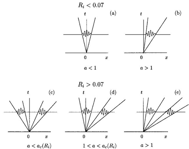
FIG. 5. Sketch of the impulse response in the  $(x, t)$  plane. For  $R_i < 0.07$  a single wave packet, (a) absolutely unstable for  $a < 1$  and (b) convectively unstable for  $a > 1$ . For  $R_i > 0.07$  behavior of the two Holmboe wave packets for  $a$  positive varying as indicated on the figure.
