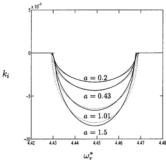
FIG. 13. Spatial growth rate of the right-going Holmboe wave versus the intrinsic frequency  $\omega_r^*$ , for  $R_i=4$  and different values of the advection parameter  $a$ ,  $a=1.5$ ,  $a=1.01$ ,  $a=0.43$ , and  $a=0.2$ . In solid curve, Holmboe branches obtained by solving the dispersion relation, in dotted curve by following the Gaster transformation (10).
