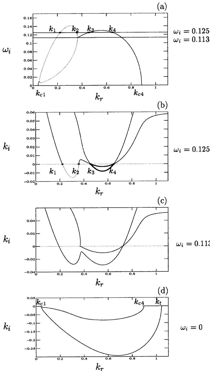
FIG. 6. In dotted curve, Kelvin-Helmholtz branches. In solid curve Holmboe branches (a) temporal growth rate  $\omega_i$  function of the wave number  $k_r$  for  $R_i=0.04$ ; spatio-temporal branches for  $R_i=0.04$  and  $a=1.1$   $\omega_r$  varies between 0 and 1.5 by small increments (b) for  $\omega_i = 0.125$ , (c) pinching of amplified branches and exchange of branches for  $\omega_i=0.113$ , and (d) hybrid spatial branches  $\omega_i=0$ .
