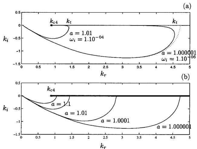
FIG. 7. (a) Comparison between the most amplified spatio-temporal branches in solid curve at small values of  $\omega_i$  and between the spatial branches  $\omega_i=0$  in dotted curve for two values of  $a$ ,  $a=1.01$  and  $a=1.000001$ . (b) Behavior of the most amplified hybrid spatial branch, Fig. 6(d), for  $R_i=0.04$  and for  $a=1.1$ ,  $a=1.01$  and  $a=1.0001$ , and  $a=1.000001$ ;  $k_{c4}$  is the neutral wave number defined on Fig. 3.
