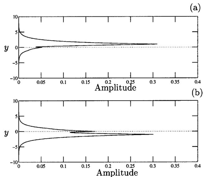
FIG. 10. Amplitude of the eigenfunction for  $R_i = 0.5$ ,  $a = 1.2$  associated with each most amplified wave number on each Holmboe branch [see Fig. 9(b)]. On (a), eigenfunction associated with the Holmboe mode traveling with the faster layer (i.e., the upper layer here) (b) eigenfunction of the most amplified wave number traveling with the lower layer.
