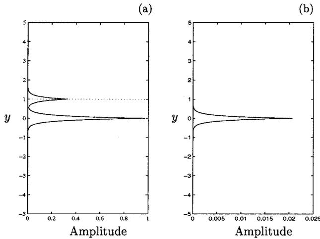
FIG. 12. (a) Amplitude of the eigenfunction associated with  $\omega_m^+$  (20) and with the most amplified wave number  $k_m$  for  $R_i=8$ . (b) Amplitude of the eigenfunction associated with the wave number  $k_0$  and with the absolute frequency  $\omega_0$  [see on Fig. 12(b)] for  $R_i=4$  and  $a=0.438$ , that means for the first convective–absolute transition.
