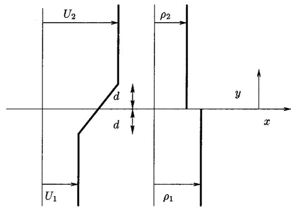
FIG. 1. Velocity and density profiles. An abrupt change in density occurs at the density interface; it is located at  $y=0$ . Abrupt changes in velocity gradient  $dU/dz$  defined the vorticity interfaces located at  $y=\pm d$ .
