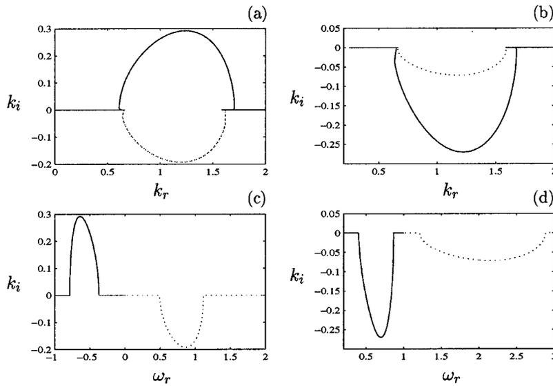
FIG. 9. Amplified spatial Holmboe branches for  $R_i = 0.5$ . In solid curve Holmboe branch associated with the lower frequency, in dotted curve Holmboe mode associated with the greater frequency; (a)  $k_i$  function of the wave number  $k_r$  for  $a=0.1$  and (b) for  $a=1.2$ ; (c)  $k_i$  function of the frequency  $\omega_r$  for  $a=0.1$ , (d) for  $a=1.2$ .
