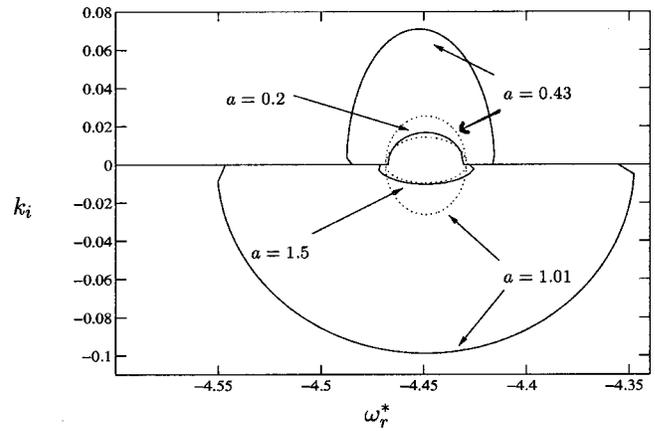
FIG. 14. Spatial growth rate for the left-going Holmboe wave versus the intrinsic frequency  $\omega_r^*$ , for  $R_i=4$  and different values of the advection parameter  $a$ ,  $a=1.5$ ,  $a=1.01$ ,  $a=0.43$ , and  $a=0.2$ . In solid curve, Holmboe branches obtained by solving the dispersion relation, in dotted curve by following the Gaster transformation (10).
