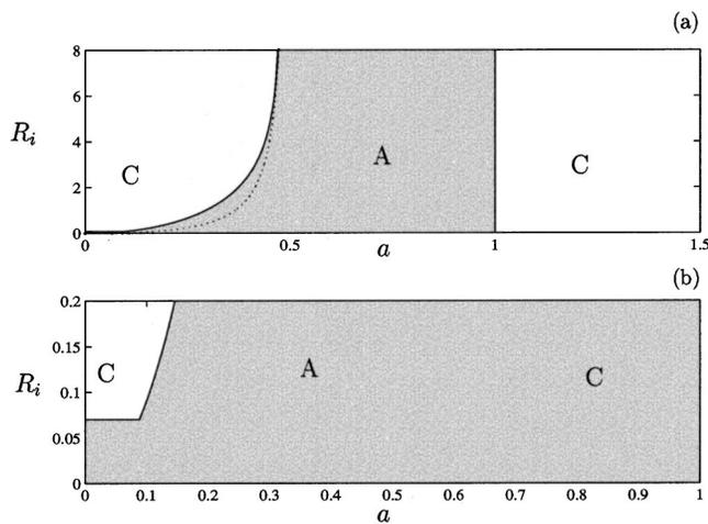
FIG. 4. (a) In light gray, **absolute instability**, A, in white **convective instability**, C, in the  $(a, R_i)$  plane. The asymptotic behavior calculated in (24) is represented by a dotted curve; (b) zoom of the absolute and convective domains for  $R_i < 0.2$ .
