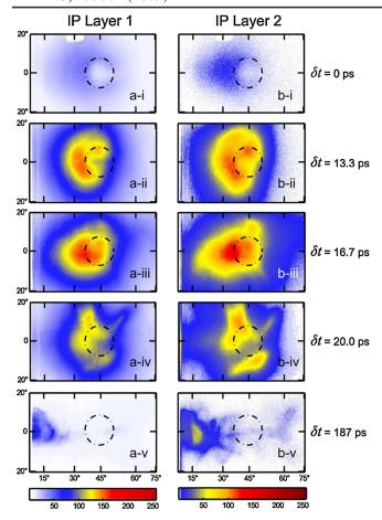
FIG. 2 (color online). Single-shot exposures of the electron beam from  $SiO_2$  plasma for different prepulse delays ( $\delta t = 0$ , 13.3, 16.7, 20.0 and 187 ps). The laser intensity is  $2.5 \times 10^{18}$  W/cm<sup>2</sup> incident along the 45° angle (marked with a dotted circle; the target surface direction is along the 90° angle). The left and right columns show electrons registered on IP layer 1 (>150 keV) and layer 2 (>350 keV), respectively.
