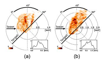
FIG. 4 (color online). Angular energy distribution of electrons outside the plasma for two different electron density scale lengths: (a)  $\lambda/5$  and (b)  $\lambda/2$ . The laser intensity is  $\sim 2 \times 10^{18} \ \text{W/cm}^2$  ( $a_o = 1$ ). The insets show a line plot of the energy distribution along the collimated beam direction.
