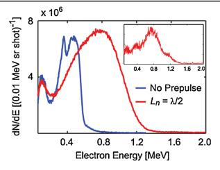
FIG. 3 (color online). Electron spectra measured along the  $\phi=36^\circ$  direction by accumulating 250 laser shots at  $I\sim2\times10^{18}~\rm W/cm^2$  for the case of no prepulse [blue (dark gray)], and a scale length of  $\simeq \lambda/2$  [red (medium gray)]. The inset shows the spectrum from a single laser shot for the optimal scale length of  $\sim \lambda/2$ .
