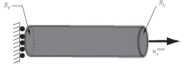
Figure 2. Meshed structure \Omega with boundary zones.
