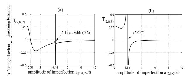
Figure 9: Type of non-linearity for (a): mode (2,0,C) and (b): (2,0,S); for an imperfection having the shape of mode (2,0,C).
