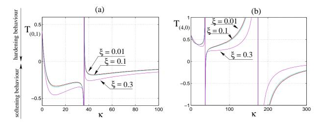
Figure 12: Type of non-linearity for (a): mode (0,1) and (b): (4,0) versus the aspect ratio  $\kappa$ . Increasing values of damping for case (ii) ( $\forall p = 1 ... N$ ,  $\xi_p = \xi$ ), are shown, with  $\xi = 0$  and 0.01 (red), 0.1 (cyan) and 0.3 (violet).
