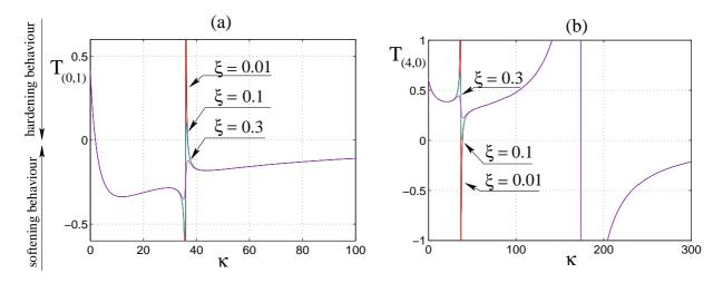
Figure 11: Type of non-linearity for (a): mode (0,1) and (b): (4,0) versus the aspect ratio  $\kappa$  of a shallow spherical shell. Increasing values of damping for case (i) ( $\forall p = 1 ... N$ ,  $\xi_p = \xi / \omega_p$ ), are shown, with  $\xi = 0$  and 0.01 (red), 0.1 (cyan) and 0.3 (violet).
