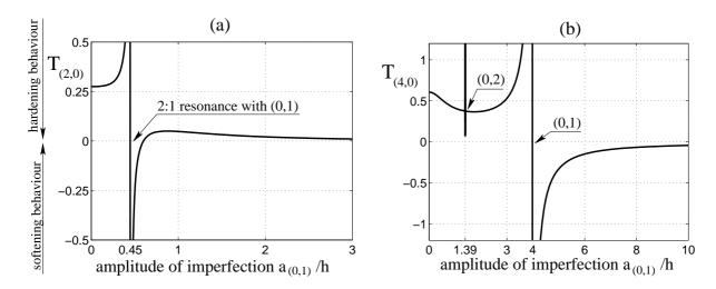
Figure 6: Type of non-linearity for (a): mode (2,0), and (b): mode (4,0), with an axisymmetric imperfection having the shape of mode (0,1).
