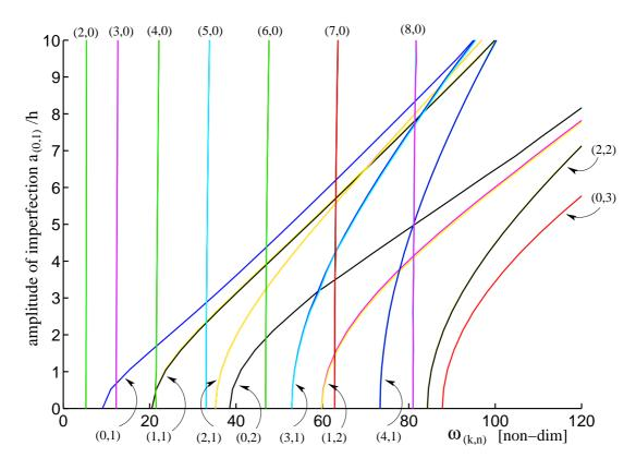
Figure 3: Non-dimensional natural frequencies  $\omega_{(k,n)}$  of the imperfect plate versus the amplitude of the imperfection having the shape of mode (0,1).
