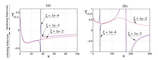
Figure 13: Type of non-linearity for (a): mode (0,1) and (b): (4,0) versus the aspect ratio  $\kappa$ . Increasing values of damping for case (iii) ( $\forall p = 1 ... N$ ,  $\xi_p = \xi \omega_p$ ), are shown, with  $\xi = 0$  and 1e-4 (black), 1e-3 (magenta) and 1e-2 (red).
