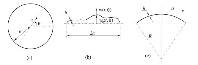
Figure 1: (a) Top view and (b) cross-section of an imperfect circular plate of radius a and thickness h. (c) The particular case of a spherical imperfection, with radius of curvature R.
