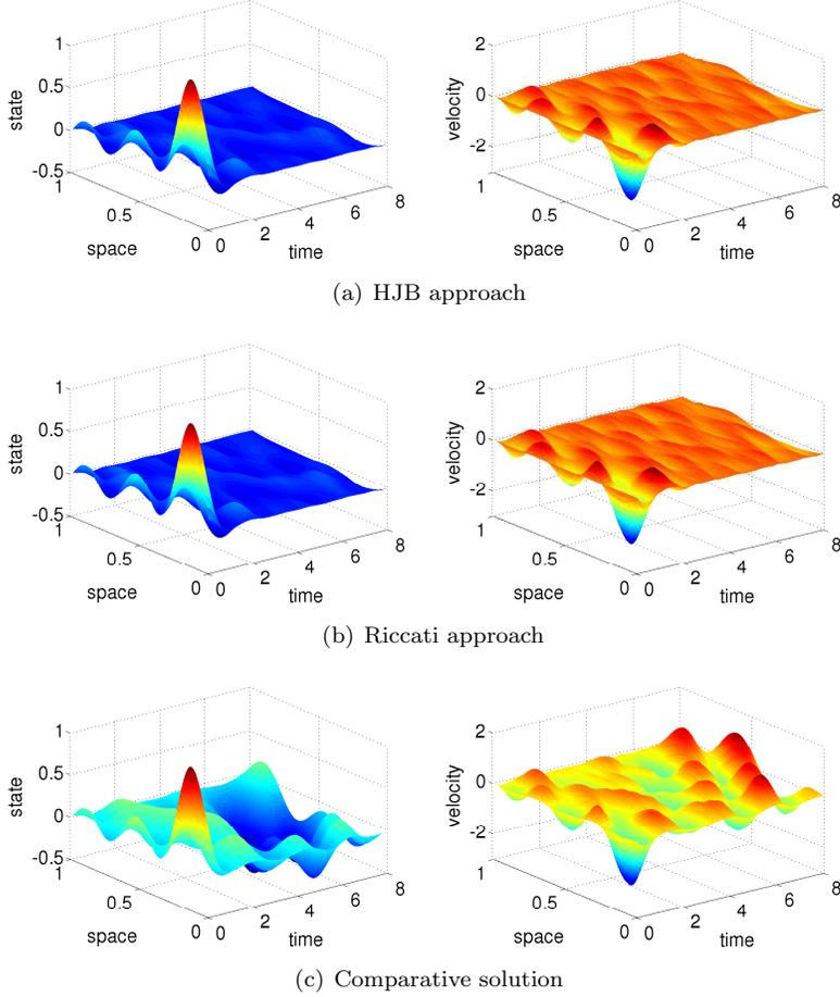
**Fig. 7.4:** Noise in the dynamics: State and velocity of the wave equation via the HJB and Riccati approach as well as the state and velocity of a noisy dynamical system controlled by the optimal control of the noise free problem, ( $\alpha = 0.01$ ).
