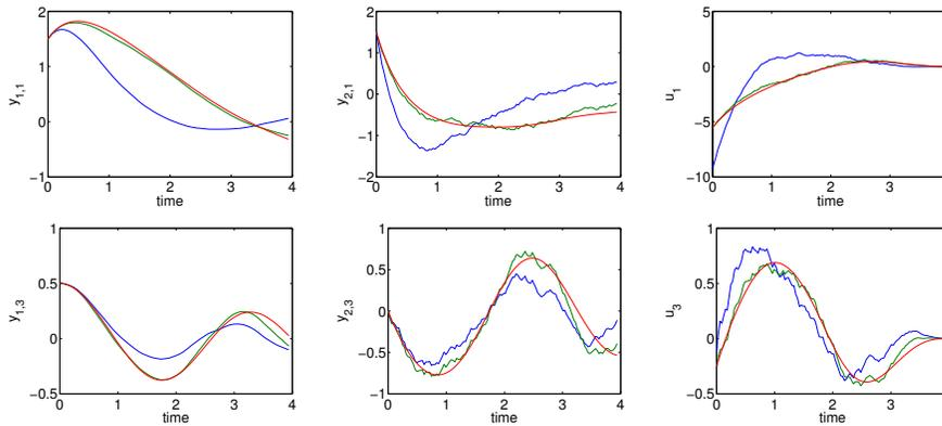
**Fig. 7.13:** Components of the trajectories and the feedback control for the HJB (blue) and linearized Riccati approach with (green) and without (red) noise for nonlinear dynamics with initial point  $y_0 = \hat{y}_0$ .
