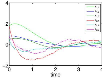
**Fig. 7.12:** Components of the trajectory for the HJB approach for nonlinear dynamics with noise
