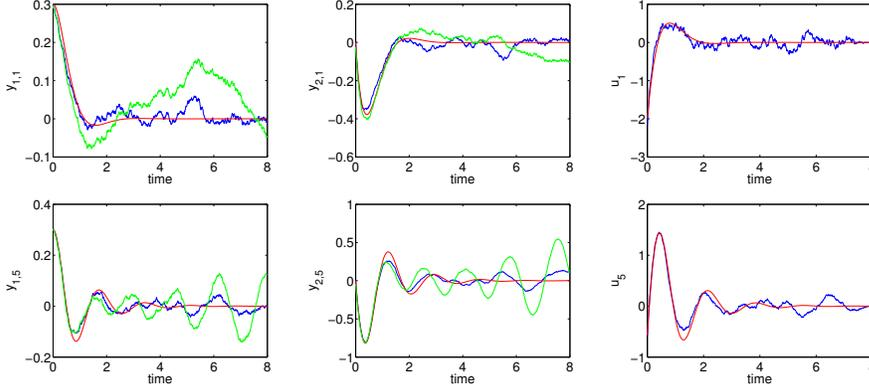
**Fig. 7.5:** Noise in the observation: Components of the trajectory and the feedback control via the HJB approach (blue) for the system with noise and via the Riccati approach (red) for the equation without noise as well as the components of the trajectory (green) when applying the optimal control of the noise free system to the perturbed system, ( $\alpha = 0.01$ )
