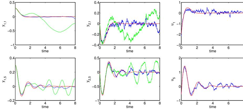
**Fig. 7.3:** Noise in the dynamics: Components of the trajectory and the feedback control via the HJB (blue) approach for the problem with noise and via the Riccati approach (red) for the equation without noise as well as the components of the trajectory (green) when applying the optimal control of the noise free system to the perturbed system, ( $\alpha = 0.01$ ).
