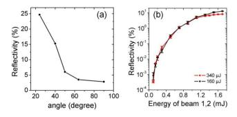
FIG. 3 (a) Reflectivity ( $R = W_4/W_3$ ) of the filament mirror as a function of angle  $\theta$  between pulse 1 and 3. Here  $W_1 = W_2 = 0.8$  mJ;  $W_3 = 170 \mu$ J. (b) Reflectivity as a function of pulse 1, 2 energy. Pulse 3 has energy of 160 and 340  $\mu$ J and is incident at an angle of 90°. The three pulses are coincident in time.
