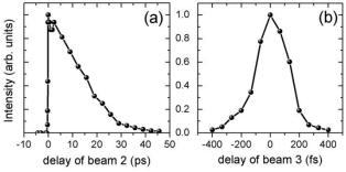
FIG. 4. (a) Signal of pulse 4 as a function of delay of filament pulse 2. Pulse 3 is incident at an angle of  $90^{\circ}$ . Pulses 1 and 3 are coincident in time. (b) The same, but delaying the pulse 3 with respect to pulses 1 and 2.
