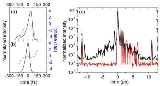
FIG. 5. Temporal profile of incident pulse 3 (a) and reflected pulse 4 (b) measured with a FROG apparatus. (c) Contrast measurement performed with a  $3\omega$  cross-correlator of laser pulse 3 before (black line) and after (red line) reflection by the filament mirror. The black arrow indicates an artifact of the correlator.
