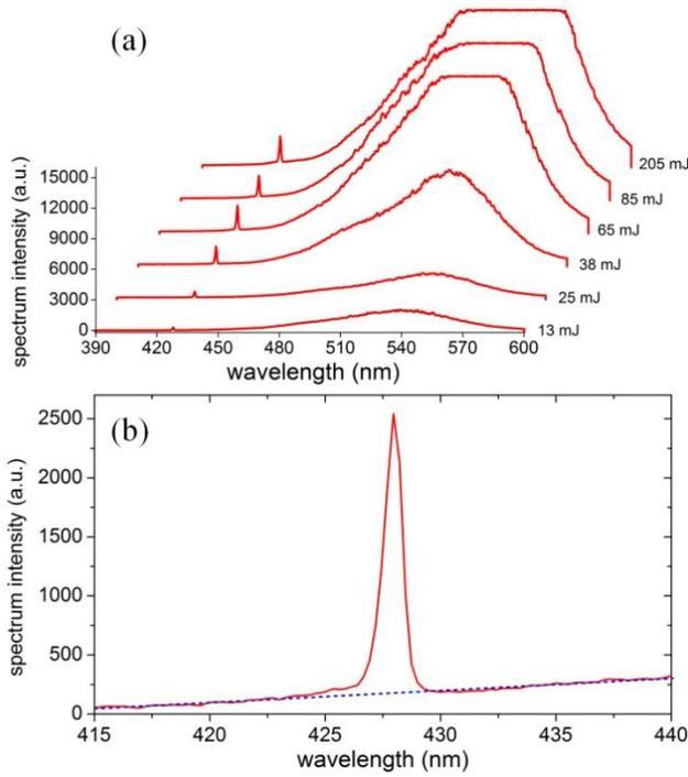
Fig. 1. (a), Spectrum of the forward emission after filamentation of laser pulses in ambient air. The focal length was 100 cm. (b), Zoomed spectrum around 428nm in the case of  $E_{in} = 65$  mJ. The dotted line shows the estimated contribution of the supercontinuum white-light.
