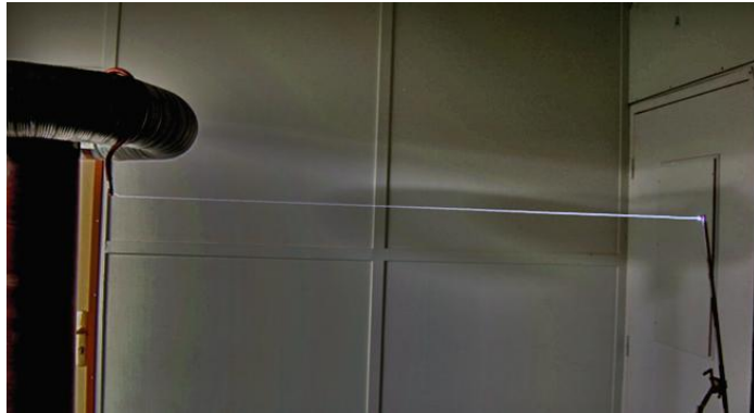
Figure 19. Photography of a Tesla guided discharge of 1.7 m. The laser beam comes from the left.
