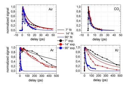
**Figure 7.** Normalized intensity of diffracted probe signal as a function of the delay  $\tau$  (ps) for crossing angles  $\varphi$  of 7°, 14° and 90° in different gases (Air, CO<sub>2</sub>, Ar and Kr). Measurements are represented by dots. Calculations are represented by solid lines.
