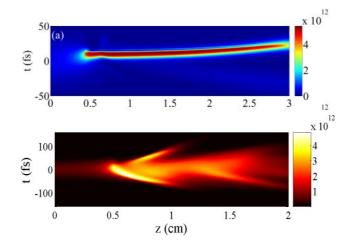
Figure 3. Numerical calculation of the pulse evolution during filamentation in silica for a femtosecond pulse with a central wavelength at  $1.6 \ \mu m$  (a) and at 800 nm (b).
