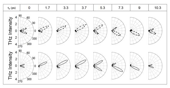
Figure 15. Evolution of emission diagrams of the THz radiation from two neighbouring filaments as a function of the temporal delay between the two laser pulses. The two filaments are separated by d = 2.4 mm. Top row: experimental results. Bottom row: calculations.
