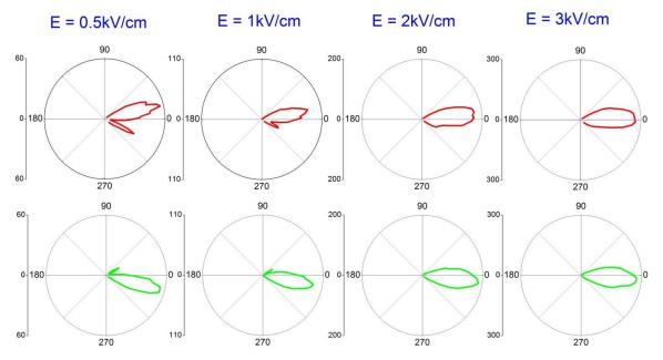
**Figure 14.** THz Radiation pattern from a laser filament in the presence of increasing transverse electric field. In the top (bottom) row, the external electric field is directed downward (upward).
