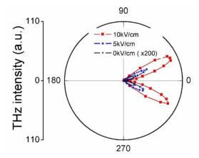
**Figure 13.** Amplification of the transition-Cherenkov THz emission. The pure transition-Cherenkov THz ( $E_{ext} = 0 \text{ kV/cm}$ ) is multiplied by a factor of 200 for visibility.
