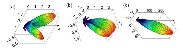
**Figure 16.** Calculated THz radiation diagram from two parallel filaments separated by 2.4 mm without time delay (a) and with a time delay  $\tau_p = 3.5$  ps (b). (c) Calculated THz radiation diagram from 16 filaments with proper time delays.
