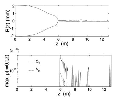
**Figure 1.** (a) Beam width of a collimated femtosecond laser pulses during filamentation propagation in air, obtained from numerical simulation. (b) The corresponding plasma density as a function of propagation distance.
