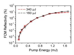
**Figure 11.** Reflectivity as a function of the pump pulses energy. Probe pulse has energy of 160 and 340  $\mu$ J and is incident at an angle of 90°. The three pulses are coincident in time.
