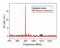
**Figure 21.** RF signal strength with (red) or without (black) the plasma column when the coupler is excited at 990 MHz. The insert corresponds to a zoom of the highlighted region around 990 MHz.
