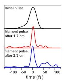
**Figure 6.** Measurement of the 1.9  $\mu$ m pulse temporal shape after propagation in the sample performed with a WIZZLER.
