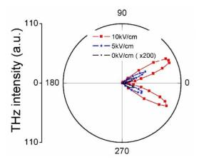
**Figure 13.** Amplification of the transition-Cherenkov THz emission. The pure transition-Cherenkov THz ( $E_{ext} = 0 \text{ kV/cm}$ ) is multiplied by a factor of 200 for visibility.
