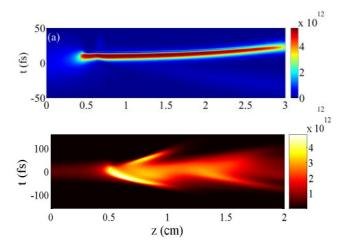
**Figure 3.** Numerical calculation of the pulse evolution during filamentation in silica for a femtosecond pulse with a central wavelength at 1.6 μm (a) and at 800 nm (b).
