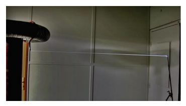
**Figure 19.** Photography of a Tesla guided discharge of 1.7 m. The laser beam comes from the left.
