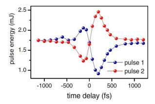
**Figure 8.** Energy exchange between two filaments crossed with an angle of 20°.
