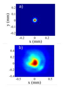
**Figure 5.** Beam profile of the laser pulse at 1.9  $\mu$ m (a) with filamentation and (b) without filamentation in the fused silica sample. Intensity scale is normalized.
