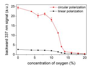
Fig. 8. Measured backward 337 nm signal from filaments in air as a function of Oxygen gas concentration, for both circular and linear polarized laser pulses. The incident pulse energy is 9.3 mJ
