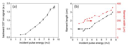
Fig. 3. (a) Backward 337 nm signal as a function of incident laser pulse energy. (b) Measured length and width of plasma as a function of pump laser energy. In both cases the pump laser is linearly polarized.
