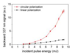
Fig. 5. Measured backward signal at 337 nm as a function of incident laser pulse energy, for both circular and linear laser polarization.
