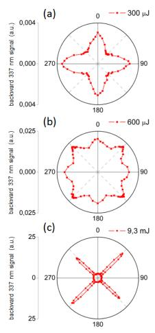
Fig. 6. Backward emission signal at 337 nm as a function of the rotation angle of the quarter-wave plate. The incident laser energy for (a), (b), (c) are 0.3 mJ, 0.6 mJ, and 9.3 mJ, respectively. Angle  $0^{\circ}$  corresponds to linearly polarized light.
