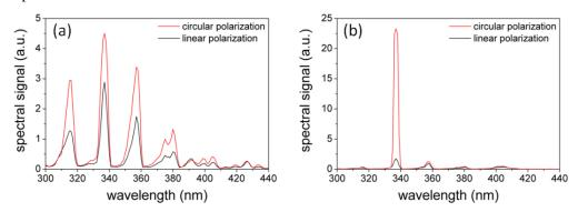
Fig. 2. Spectra of (a) transverse fluorescence and (b) backward UV emission for circular and linear laser polarization. The incident laser pulse energy is 9.3 mJ.
