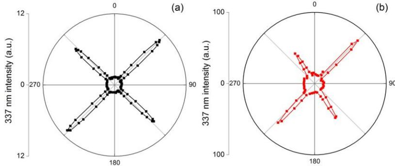
Fig. 7. Dependence of the backward ASE (a) and the seeded backward stimulated radiation (b) as a function of the rotation angle of the quarter-wave plate. The angles  $\phi = 90^\circ \times m$  correspond to linearly polarized laser, with  $m = 0, 1, 2, 3$ . The angles  $\phi = 45^\circ + 90^\circ \times m$  correspond to circularly polarized laser.
