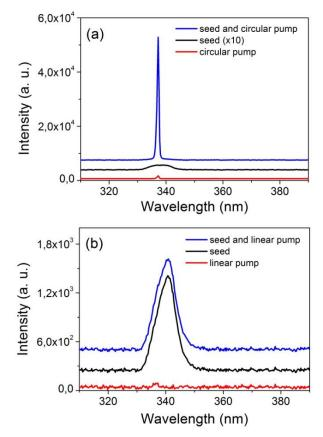
Fig. 3. Spectra of the backward emission with circularly (a) and linearly (b) polarized pump pulsed at 800 nm. The spectra of the seed pulses and those of the backward emission from the pump pulses are also presented for comparison. In (a), the spectrum of the seed pulse is magnified by a factor of 10 for visibility.
