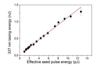
Fig. 6. Energy of the amplified 337 nm emission in the backward direction as a function of the seed pulse energy.
