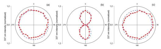
Fig. 4. Polarization of the ASE (a), the seeded backward stimulated emission with linearly (b) and circularly (c) polarized seed pulses at 337 nm. The dots present the experimental results and the dashed lines denote the theoretical fitting.
