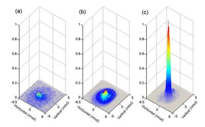
Fig. 5. Spatial profile of the backward ASE (a), the seed pulse (b), and the amplified 337 nm radiation (c). The opening angle of each panel is 12.5 mrad  $\times$  10 mrad.
