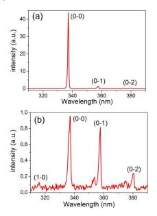
Fig. 2. Backward emission spectrum with circularly (a) and linearly (b) polarized pump pulses. The numbers in the parenthesis denote the vibration quantum number of the initial and final states of the transition.
