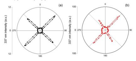
Fig. 7. Dependence of the backward ASE (a) and the seeded backward stimulated radiation (b) as a function of the rotation angle of the quarter-wave plate. The angles  $\varphi = 90^{\circ} \times m$  correspond to linearly polarized laser, with m = 0, 1, 2, 3. The angles  $\varphi = 45^{\circ} + 90^{\circ} \times m$  correspond to circularly polarized laser.
