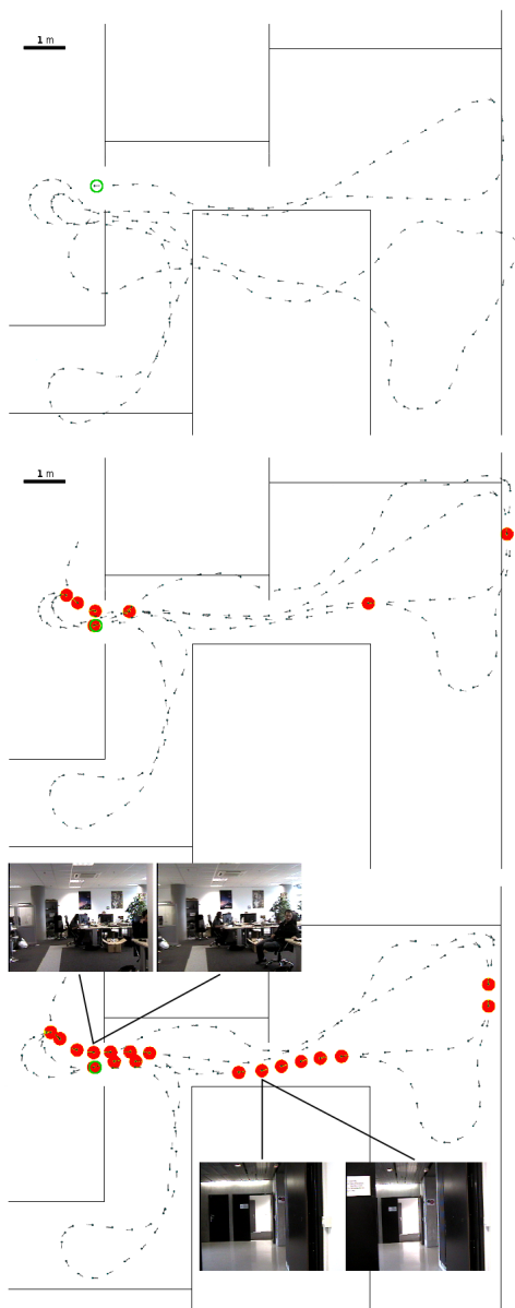
Fig. 10. Gostai sequence: example of topo-metric mapping results a. raw odometry, b. topo-metric map using the loop-closure framework from [2] (7 loop-closures) c. map using the proposed model (18 loop-closures).
