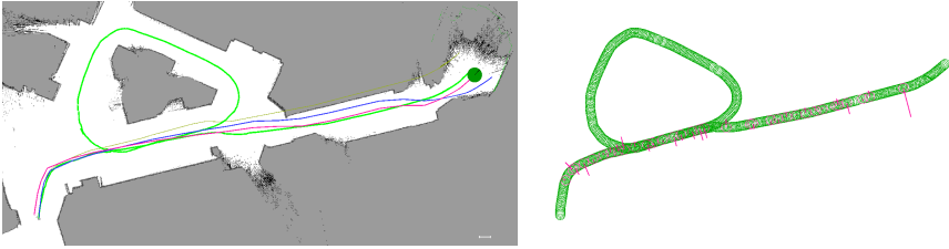
Fig. 13. Example of vision based path following. Green circles represent learned places and magenta circles show the loop-closure locations detected during the navigation. The line in the middle of the magenta circles corresponds to the x-axis translation computed from the matching images.
