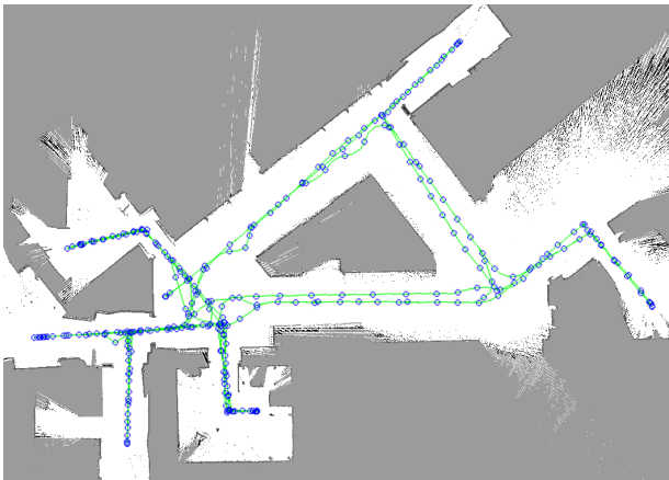
Fig. 12. A large topo-metric map in a 6 rooms environment showing the consistency of the produced map ('6 rooms' sequence, 1325 images, 352 loop-closures).
