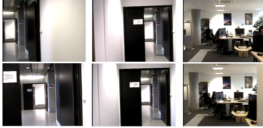
Fig. 6. Examples of loop-closure acceptance: First column: match accepted after epipolar geometry validation at a door crossing (Gostai sequence) with more than 1 meter difference between robot positions. Second and third columns : matches accepted using the new validation proposed in this paper with 5cm error.
