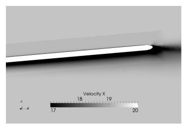
**FIGURE 8.** VELOCITY IN THE X-DIRECTION, CYLINDER IN NEAR AXIAL FLOW WITH AN ANGLE  $\alpha=5^\circ$ , LONGITUDINAL SECTION
