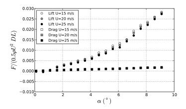
**FIGURE 5**. EXPERIMENTAL LIFT AND DRAG COMPONENT OF THE NORMAL FORCE VS. INCLINATION ANGLE [10]
