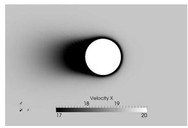
**FIGURE 9.** VELOCITY IN THE X-DIRECTION, CYLINDER IN NEAR AXIAL FLOW WITH AN ANGLE  $\alpha=5^\circ$ , TRANSVERSE SECTION
