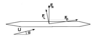
**FIGURE 1**. VELOCITY IN THE X-DIRECTION, CYLINDER IN NEAR AXIAL FLOW WITH AN ANGLE  $\alpha=5^\circ$
