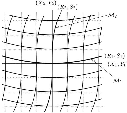
*Fig. 1: Sketch of the phase space in the vicinity of the origin. Orthogonal lines represent the linear modal basis. Curved lines tangent at the origin represents the invariant manifolds, i.e. the NNMs. A curved grid is also represented, in which the normal dynamics will be expressed.*
