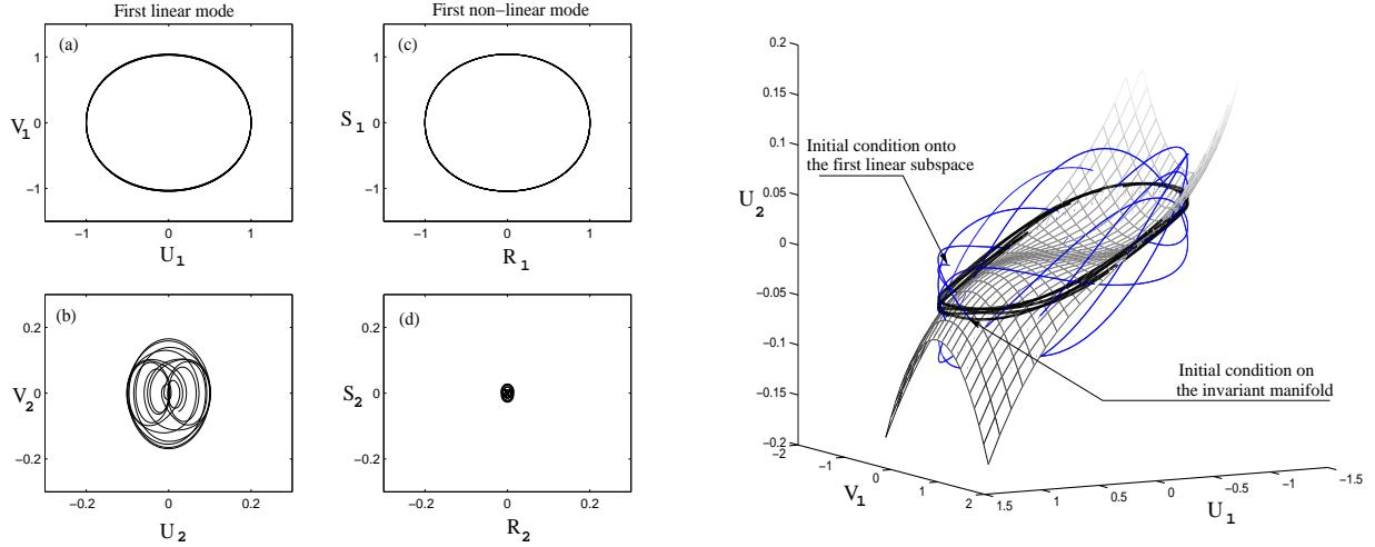
*Fig. 3: (a)-(d): projections onto linear and non-linear subspaces of a motion initiated along the first linear mode(a)-(b) ; and along the first non-linear mode (c)-(d). Representation of the two precedent simulations in  $(U_1, V_1, U_2)$  space, showing the invariance property for the first NNM.*
