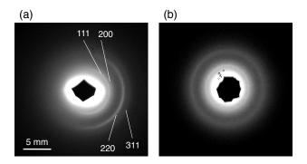
FIG. 3: Electron diffraction patterns from a 10 nm thick polycrystalline Al foil. (a) The diffraction pattern is assymetric because of a spatial chirp in the electron beam. (b) Symmetric diffraction pattern obtained by removing the spatial chirp on the electron beam.
