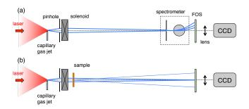
FIG. 1: (a) Experimental set-up for electron beam characterization with an electron spectrometer. (b) Set-up for diffraction. The solenoid is placed 60 mm after the electron source, the distance between the sample and the scintillator (FOS) is 220 mm.
