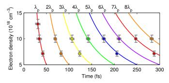
Figure 4. (Color online) Average positions of the Fourier peaks for different plasma densities (o) are compared to multiples of the plasma wave period (lines). Horizontal errorbars denote the standard deviation over the complete dataset. Vertical errorbars is an estimate of the uncertainty in plasma density.
