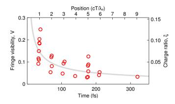
Figure 3. (Color online) Fringe visibility for sinusoidal oscillation that contained only one significant peak in the Fourier Transform, as function of the position of that peak. The charge ratio  $\xi = q_n/q_o$  is calculated from the visibility using Eq. 2 in the limit where both bunches have similar shapes and energy distributions. The measurements were performed using CPI for  $n_e = 10 \times 10^{18}$  cm<sup>-3</sup>.
