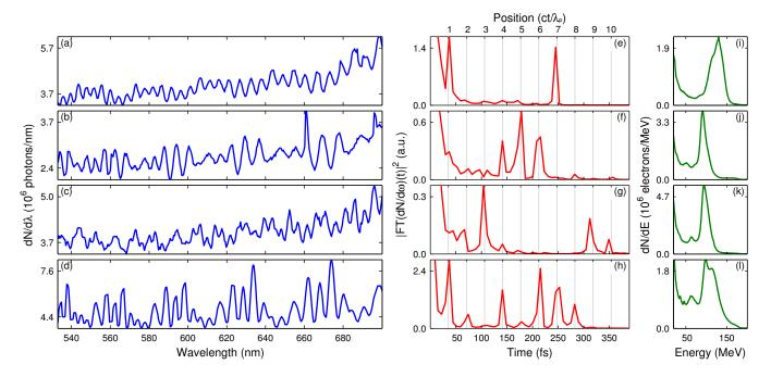
Figure 2. (Color online) Selected examples of complex CTR modulations, obtained using CPI for  $n_e = 10 \times 10^{18}$  cm<sup>-3</sup> and  $\lambda_p = 10.6 \mu$ m. Three panels on each row represent one measurement. (a–d): CTR spectra. (e–h): Fourier transform of the CTR spectra. (i–l): Corresponding electron spectra.
