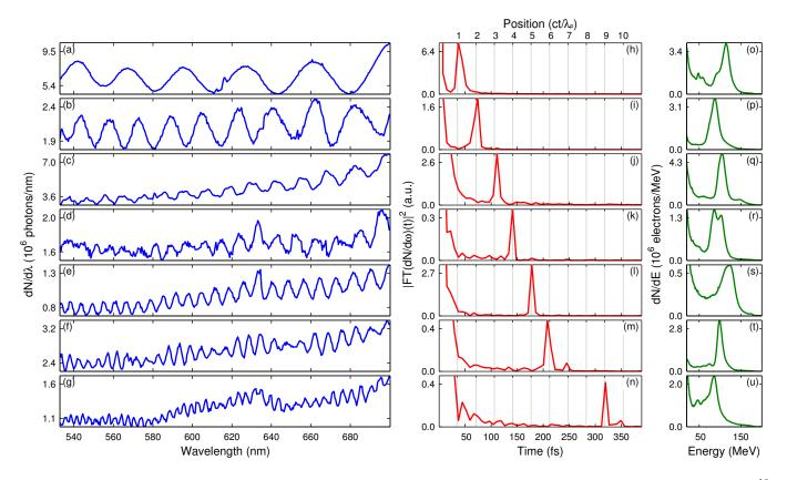
Figure 1. (Color online) Selected and sorted examples of sinusoidal CTR modulations, obtained using CPI for  $n_e = 10 \times 10^{18}$  cm<sup>-3</sup> and  $\lambda_p = 10.6 \,\mu\text{m}$ . Three panels on each row represent one measurement. (a–g): CTR spectra. (h–n): Square amplitude of the Fourier transform of the CTR spectra. (o–u): Corresponding electron spectra.
