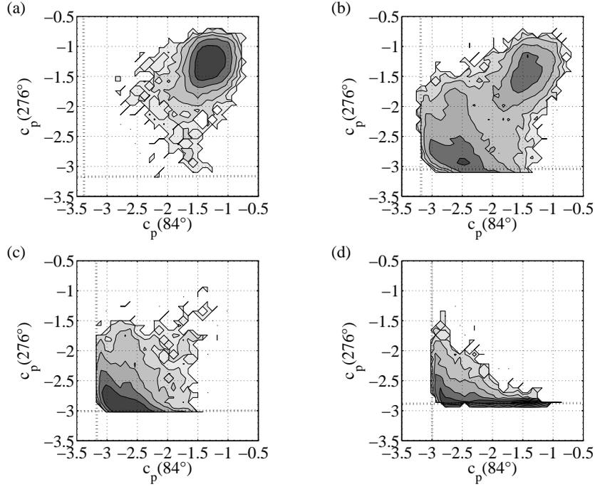
FIG. 23. Joint probability density function of  $c_p(84^\circ)$  and  $c_p(276^\circ)$  for (a)  $Re = 3.47 \times 10^5$ , (b)  $Re = 3.61 \times 10^5$  (c)  $Re = 3.67 \times 10^5$  and (d)  $Re = 3.74 \times 10^5$ . Vertical and horizontal dashed lines show the saturated value introduced by the higher limit of the pressure scanner.
