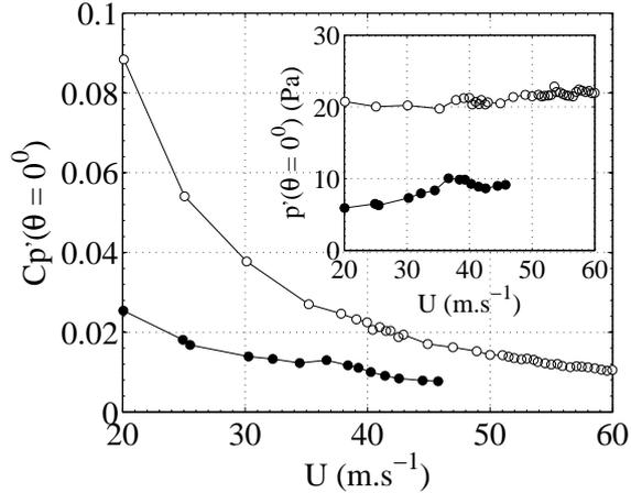
FIG. 3. Fluctuating pressure coefficient  $Cp'$  as defined in Eq. 1 at the front head of the cylinder ( $\theta = 0^\circ$ ) as described in Fig. 4 vs. the velocity in the wind tunnel. Empty symbols refer to the wide range pressure scanner which is used to obtain the result of the present work (section IIB) and filled symbols correspond to a more accurate pressure scanner but having a smaller range. The inserted graphics display the corresponding pressure.
