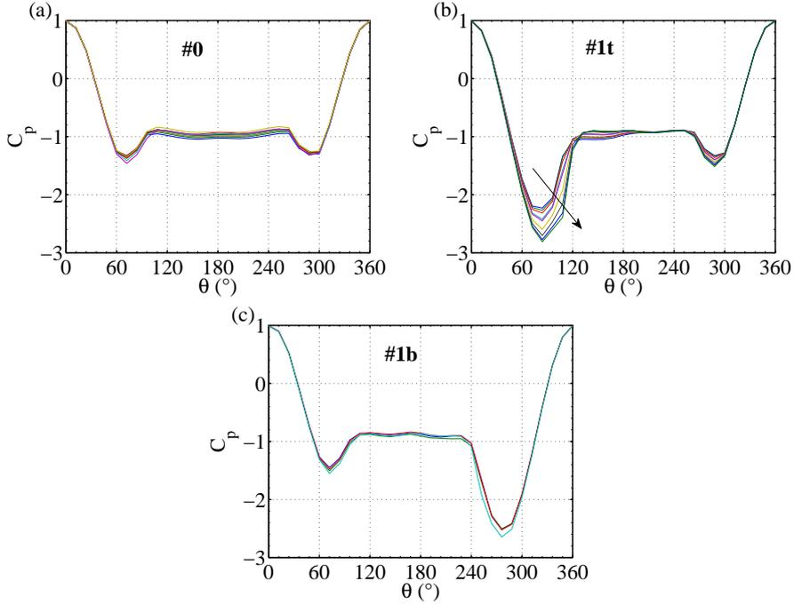
FIG. 18. Pressure distributions of the conditional statistics #0 (a), #1t (b), #1b (c) for Reynolds numbers in the range  $2.99 \times 10^5 < Re < 3.45 \times 10^5$  during the primary reattachment of the antisymmetric scenario. Arrows are indicating the hierarchy of the curves for increasing  $Re$ .
