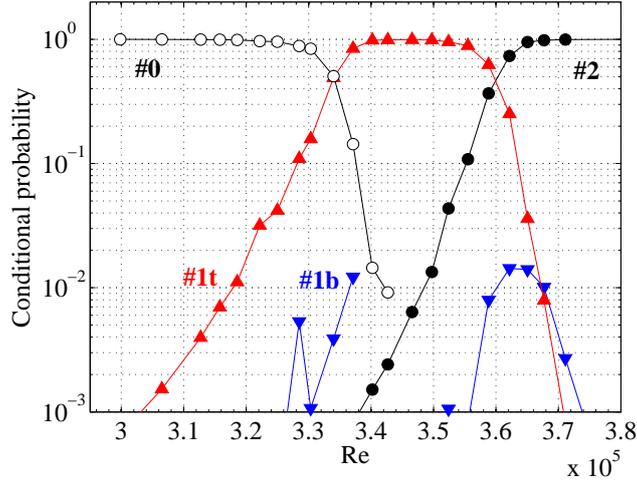
FIG. 17. Probability of the conditional statistics of states #0, #1b, #1t and #2 during the asymmetric reattachment process.
