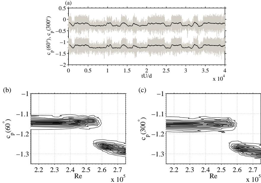
FIG. 13. Signals with large fluctuations in (a) are the time series for the two symmetric angular positions  $c_p(60^\circ, tU/d)$  (bottom) and  $c_p(300^\circ, tU/d)$  (top) at  $Re = 2.56 \times 10^5$ . For clarity,  $c_p(300^\circ, t)$  is artificially shifted by 1. Thin lines are the low pass filtered time series. Probability functions of the filtered time series of pressure (b)  $c_p(60^\circ)$  and (c)  $c_p(300^\circ)$  vs.  $Re$ .
