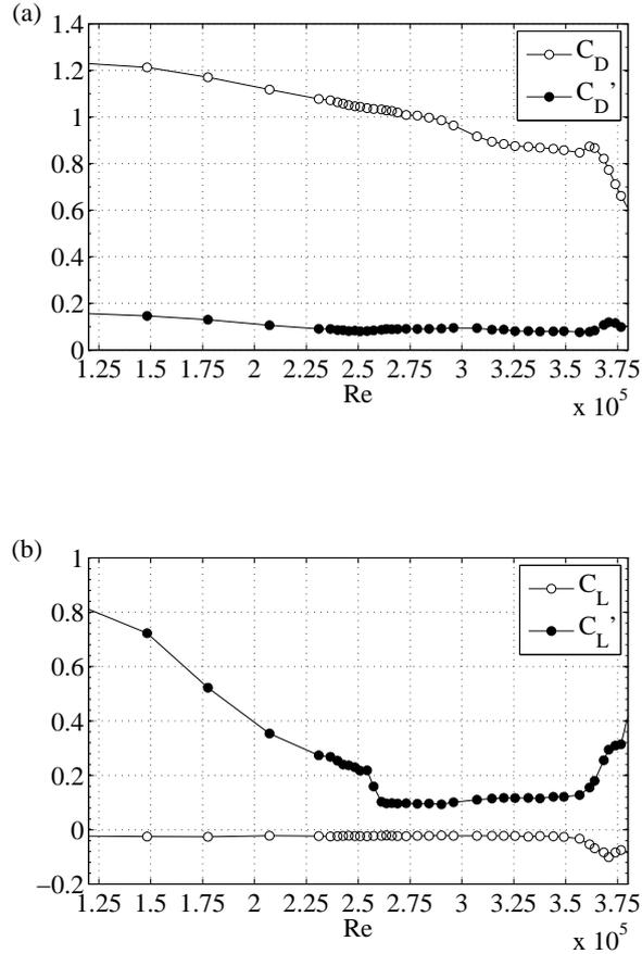
FIG. 9. Sectional mean and fluctuations drag and lift vs.  $Re$  computed from the data of the symmetric reattachments in Fig. 7.
