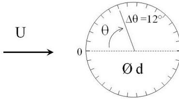
FIG. 4. Central section of the cylinder. Each tick symbolizes a hole of 1 mm dedicated for wall pressure measurements. The side  $0^\circ < \theta < 180^\circ$  will be referred as the top side in the text, the side  $180^\circ < \theta < 360^\circ$  as the bottom side.
