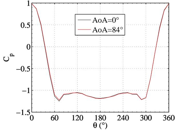
FIG. 5. Comparison of the angular distribution of the pressure coefficient for the subcritical regime at  $Re = 1.85 \times 10^5$  obtained for both angles of attack  $0^\circ$  and  $84^\circ$  of the cylinder.
