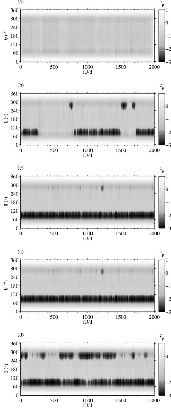
FIG. 15. Space time diagrams of the pressure distribution  $c_p(\theta, tU/d)$  for (a)  $Re = 2.99 \times 10^5$ , (b)  $Re = 3.37 \times 10^5$ , (c)  $Re = 3.49 \times 10^5$ , (d)  $Re = 3.59 \times 10^5$  and (e)  $Re = 3.78 \times 10^5$ .
