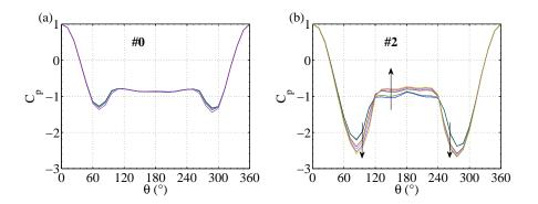
FIG. 25. Pressure distributions of the conditional statistics #0 (a), #2 (b) for Re in the range  $3.55 \times 10^5 < Re < 3.68 \times 10^5$  during the reattachments of the symmetric scenario. Arrows are indicating the hierarchy of the curves for increasing Re.
