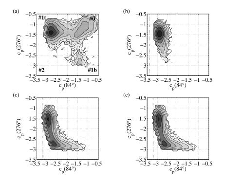
FIG. 16. Joint probability density function of  $c_p(84^\circ)$  and  $c_p(276^\circ)$  for (a)  $Re = 3.37 \times 10^5$ , (b)  $Re = 3.49 \times 10^5$ , (c)  $Re = 3.59 \times 10^5$  and (d)  $Re = 3.78 \times 10^5$ . Vertical and horizontal dashed lines show the saturated value introduced by the higher limit of the pressure scanner.
