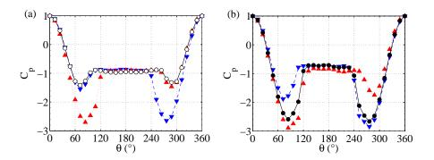
FIG. 20. Pressure distributions of the conditional statistics during the two lift fluctuation crisis of the asymmetric reattachment scenario, (a) at  $Re = 3.35 \times 10^5$  and (b) at  $Re = 3.59 \times 10^5$ . See Fig. 17 for symbols legend.
