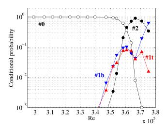
FIG. 24. Probabilities of the conditional statistics #0, #1b, #1t and #2 during the symmetric reattachment process.
