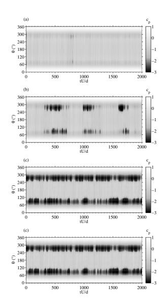
FIG. 22. Space time diagrams of the pressure distribution  $c_p(\theta, tU/d)$  for (a)  $Re = 3.47 \times 10^5$ , (b)  $Re = 3.61 \times 10^5$  (c)  $Re = 3.67 \times 10^5$  and (d)  $Re = 3.74 \times 10^5$ .
