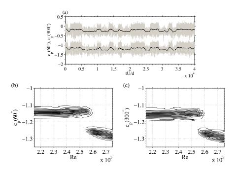
FIG. 13. Signals with large fluctuations in (a) are the time series for the two symmetric angular positions  $c_p(60^\circ, tU/d)$  (bottom) and  $c_p(300^\circ, tU/d)$  (top) at  $Re = 2.56 \times 10^5$ . For clarity,  $c_p(300^\circ, t)$ is artificially shifted by 1. Thin lines are the low pass filtered time series. Probability functions of the filtered time series of pressure (b)  $c_p(60^\circ)$  and (c)  $c_p(300^\circ)$  vs. Re.
