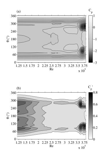
FIG. 7. Mean (a) and rms value (b) of the angular distribution of the pressure coefficient vs. Re. The only difference with the experiment in Fig. 6 is that the cylinder has been rotated by an angle of  $84^{\circ}$ .
