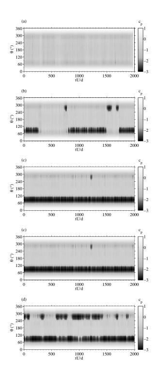
FIG. 15. Space time diagrams of the pressure distribution  $c_p(\theta, tU/d)$  for (a)  $Re = 2.99 \times 10^5$ , (b)  $Re = 3.37 \times 10^5$ , (c)  $Re = 3.49 \times 10^5$ , (d)  $Re = 3.59 \times 10^5$  and (e)  $Re = 3.78 \times 10^5$ .
