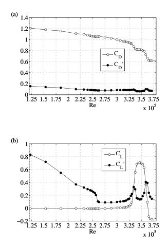
FIG. 8. Sectional mean and fluctuations drag and lift vs. *Re* computed from the data of the asymmetric reattachments in Fig. 6.
