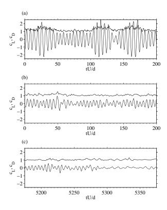
FIG. 11. Drag,  $c_D$  (thick line) and lift,  $c_L$  (thin line) coefficients corresponding to Fig. 10 for (a)  $Re = 1.22 \times 10^5$ , (b)  $Re = 2.45 \times 10^5$  and (c)  $Re = 2.56 \times 10^5$ .
