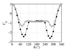
FIG. 26. Pressure distributions of the conditional statistics #0 and #2 during the lift fluctuation crisis of the symmetric reattachment scenario at  $Re = 3.61 \times 10^5$ . See Fig. 17 or 24 for symbols legend.
