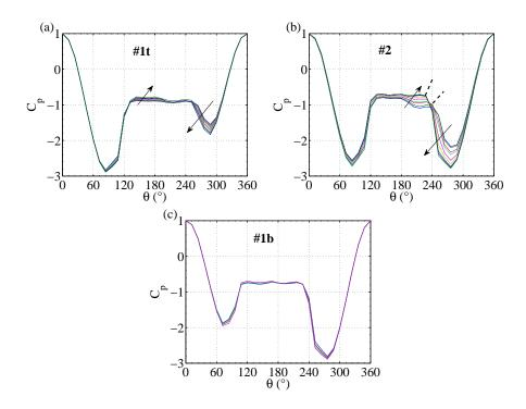
FIG. 19. Pressure distributions of the conditional statistics #1t (a), #2 (b), #1b (c) for Reynolds numbers in the range  $3.5 \times 10^5 < Re < 3.8 \times 10^5$  during the secondary reattachment of the antisymmetric scenario. Arrows are indicating the hierarchy of the curves for increasing *Re*. Dashed lines help to locate the separation angles.
