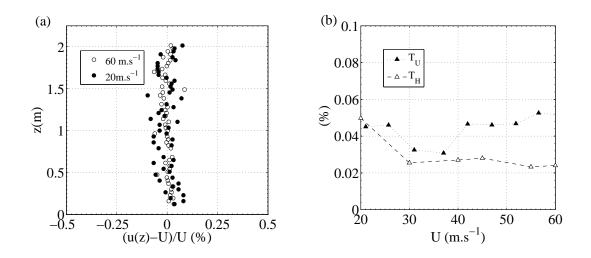
FIG. 2. Vertical mean velocity profiles in the test area for wind speeds of  $U = 60 \text{ m.s}^{-1}$  and  $U = 20 \text{ m.s}^{-1}$  (a). Turbulent intensity at mid height  $T_U$  and flow homogeneity  $T_H$  measured from the vertical mean velocity profiles (b).
