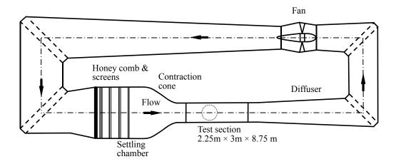
FIG. 1. Aerodynamic layout of the National Wind Tunnel Facility (NWTF).
