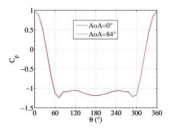
FIG. 5. Comparison of the angular distribution of the pressure coefficient for the subcritical regime at  $Re = 1.85 \times 10^5$  obtained for both angles of attack 0° and 84° of the cylinder.
