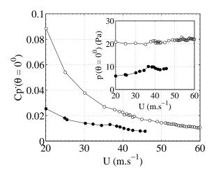
FIG. 3. Fluctuating pressure coefficient Cp' as defined in Eq. 1 at the front head of the cylinder  $(\theta = 0^{\circ})$  as described in Fig. 4 vs. the velocity in the wind tunnel. Empty symbols refer to the wide range pressure scanner which is used to obtain the result of the present work (section IIB) and filled symbols correspond to a more accurate pressure scanner but having a smaller range. The inserted graphics display the corresponding pressure.
