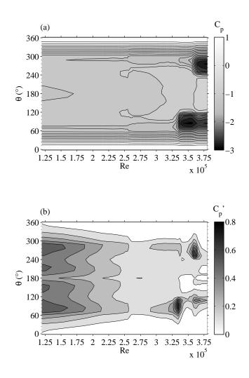
FIG. 6. Mean (a) and rms value (b) of the angular distribution of the pressure coefficient vs. Re. In (a) the exterior iso- $C_p$  line is 0.8 with intervals of 0.2. In (b) the exterior iso- $C'_p$  line is 0.1 with intervals of 0.1.
