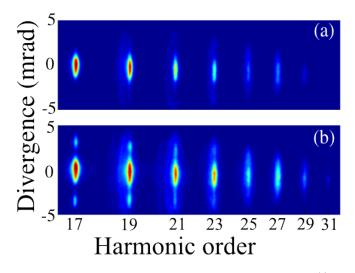
Figure 2. Spatially resolved harmonic spectrum generated in N<sub>2</sub> at  $1.5 \times 10^{14}$  W/cm<sup>2</sup>, with isotropic molecular alignment (a) and at  $\Delta t = 4.1$  ps (b).
