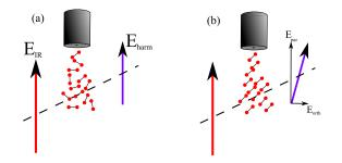
**Figure 4.** Principle of polarization resolved spectroscopy. In an isotropic medium, the harmonic polarization is parallel to the laser field (a). In an anisotropic medium this is in general not the case and an orthogonal electric field component can be produced (b).
