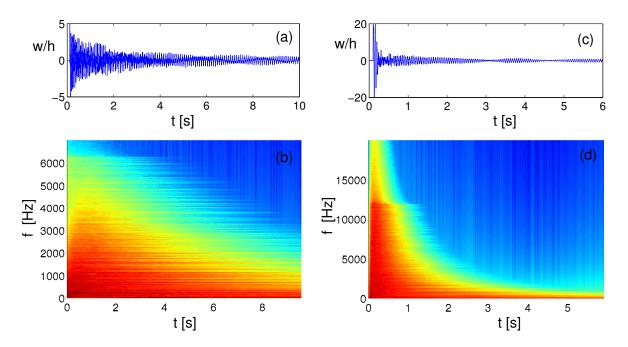
Figure 1: Time series and spectrograms of two simulated strongly nonlinear vibrations. (a)-(b): rectangular plate, (c)-(d): circular plate.
