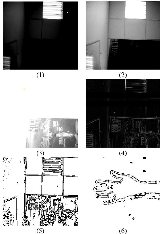
**Figure 3. Acquisition and processing within the programmable retina: (1) short exposure acquisition  $B_t$ . (2) medium exposure acquisition  $M_t$ . (3) long exposure acquisition  $D_t$ . (4) maximum of the morphological gradient over the three acquisitions  $G_t^B$ . (5) binary contours  $C_t$ . (6) moving contours detected  $E_t$ .**
