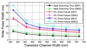
Fig.9. Comparison of writing "1" error rates between our model and Fig. 7 (b) of [25].
