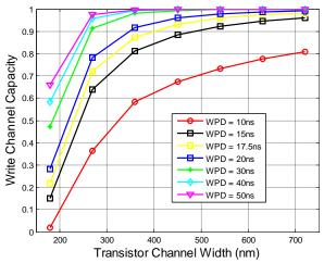
Fig.15. STT-MRAM write channel capacities with different transistor widths and different WPDs
