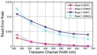
Fig.10. Reading failure rate for different transistor widths.
