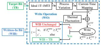
Fig.3. Block diagram of thewrite operation channel.
