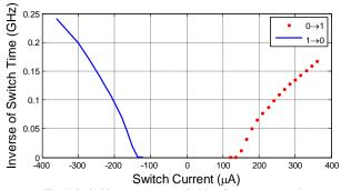
Fig.4. Switching current to switching frequency mapping.
