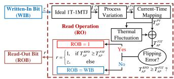
Fig.6. Block diagram of the read operation channel.
