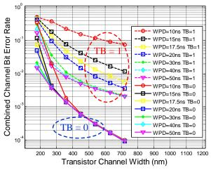
Fig.21. STT-MRAM written-in bits (WIBs) distributions with different transistor widths and different WPDs (RPD = 5ns).
