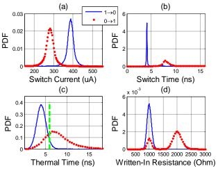
Fig.11. STT-MRAM write operational channel (transistor size = 540 nm, WPD = 10 ns).
