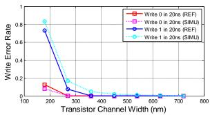
Fig.8. Write error rate for a 20 ns writing pulse width.
