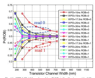
Fig.19. STT-MRAM read-out bits (ROBs) distributions with different transistor widths and different WPDs (RPD = 5ns).
