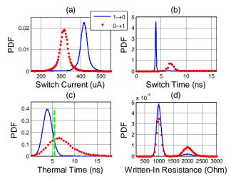
Fig.12. STT-MRAM write operational channel (transistor size = 720nm, WPD = 5.5 ns).
