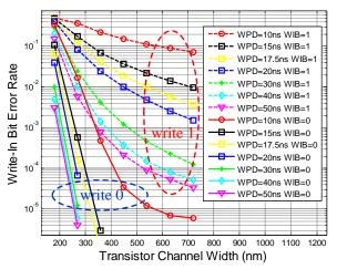
Fig.14. STT-MRAM write-in bit error rates with different transistor widths and different WPDs.
