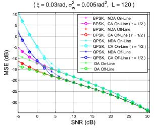
Fig. 3 HCRBs in the center of the block (i = 60) for BPSK and QPSK. ( $\xi = 0.03$ rad,  $\sigma_w^2 = 0.005$ rad<sup>2</sup> L = 120)
