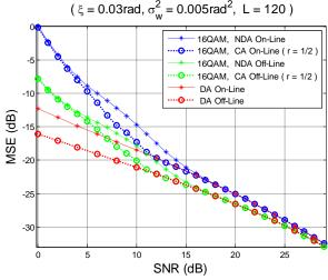
Fig. 2 HCRBs in the center of the block (l = 60) for a 16QAM.
