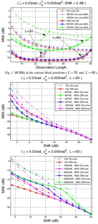
Fig. 2 HCRBs in the center of the block (l = 30) for various constellations.
