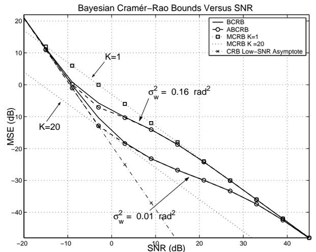
Fig. 2. Comparison between Bayesian CRBs and Asymptote-based CRBs for two different phase noise variances  $\sigma_w^2 = 0.01 \text{ rad}^2$  and  $\sigma_w^2 = 0.16 \text{ rad}^2$ .
