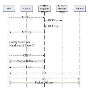
Fig. 3. E-HCF Procedure (E-HCF original router is an attached router with an E-HCF function; the E-HCF distant/remove router is a router with who an E-HCF original router can communicate)
