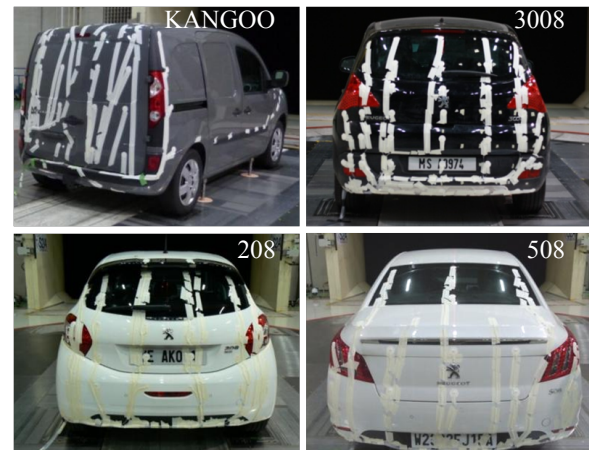
Figure 1 Rear view of the four tested vehicles with pressure measurements installation. The pressure taps location will be denoted by filled black circles in Fig. 5, 6, 7.
