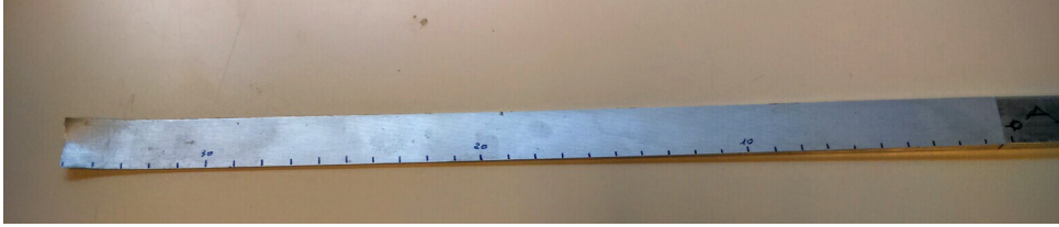
Figure 1: Extremity of the ABH beam. The length of the variable thickness region is 35 cm.
