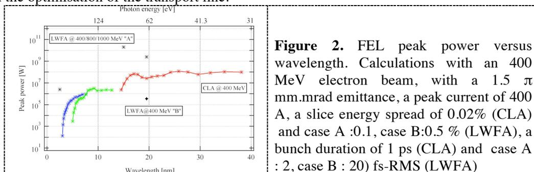
**Figure 2.** FEL peak power versus wavelength. Calculations with an 400 MeV electron beam, with a  $1.5 \pi$  mm.mrad emittance, a peak current of 400 A, a slice energy spread of 0.02% (CLA) and case A :0.1, case B:0.5 % (LWFA), a bunch duration of 1 ps (CLA) and case A : 2, case B : 20) fs-RMS (LWFA)
