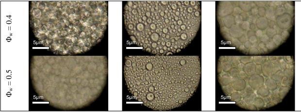
Figure 3: Effect of the OWR on the morphology of the emulsions.
