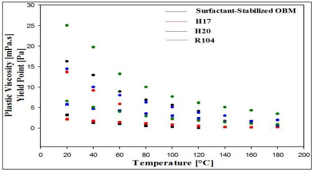
Figure 11: Effect of temperature on the rheology o drilling fluids -•- Plastic Viscosity and -**-** Yield Stress
