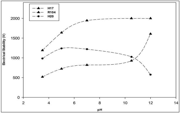
Figure 5: Effect of pH of the aqueous phase on the stability of the emulsions prepared.
