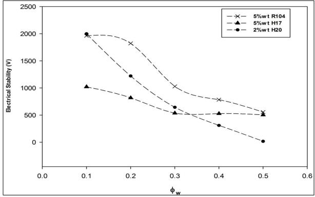
Figure 4: Effect of the water phase volume fraction on the electrical stability measurements.
