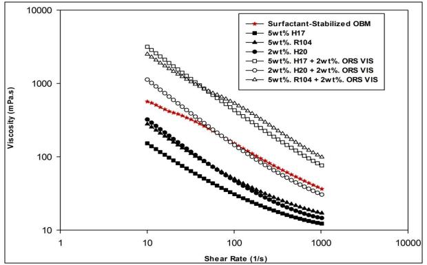
Figure 8: Flow curves of various samples prepared compared to surfactant-stabilized OBM.
