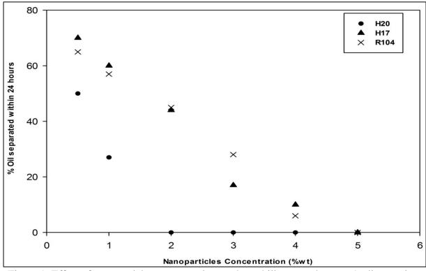
Figure 1: Effect of nanoparticles concentration on the stability to coalescence/sedimentation of the emulsions prepared.
