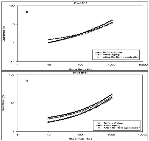
Figure 9: Flow curves of all samples prepared without clay particles showing the effect of aging and remixing on the rheological properties. (a) 2 wt.% H20 (b) 5 wt.% H17 and (c) 5 wt.% R104.
