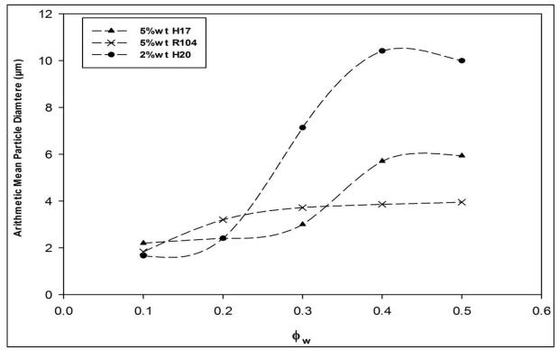
Figure 2: Variation of the arithmetic mean particle diameter with the water phase volume fraction for all three nanoparticles types.
