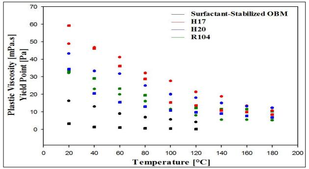
Figure 12: Effect of temperature on samples prepared with clay particles -•- Plastic Viscosity and -=- Yield Stress
