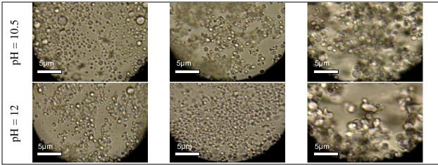
Figure 6: Effect of changing the pH of the aqueous phase on the morphology (droplet size distribution) of the emulsions.
