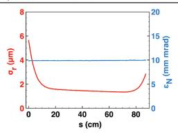
**Figure 10.** Beam spot size variation (red curve) and the emittance variation (blue line) throughout the plasma with matching sections. Values are full projections of the trailing bunch. The vacuum waist size occurs at s=0 cm and the injected bunch has a normalized emittance of  $10~\mu m$ .
