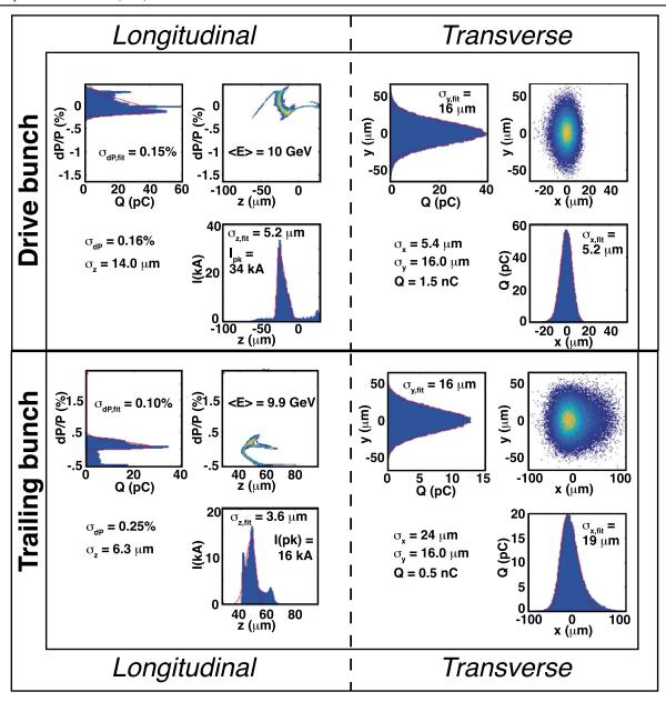
**Figure 6.** Results of 6D particle tracking, shown at the interaction point (IP), after tracking the particles from the RF gun to the IP (entrance to the plasma). Drive (witness) beams have x by y emittances of  $7.2 \times 3.2 \, \mu \text{m}$  ( $7.4 \times 3.0 \, \mu \text{m}$ ) which, for this simulation, have about twice the peak current in both bunches with respect to the minimum performance initially requested by PWFA experimentalist via 3D PIC simulations (see table 1).
