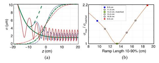
**Figure 9.** (a) An example of the determination of incoming beam parameters to match a particular profile (heavy green lines, see text) and the betatron oscillations of that same incoming beam if the profile were to change (red and dark-blue lines). (b) A summary of the maximum betatron spot size within the plasma normalize to the matched size for six profiles, three of which are shown in (a).
