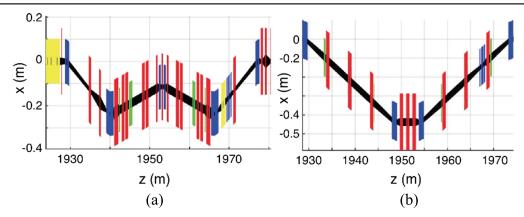
**Figure 5.** Existing final electron compression chicane (a) and its redesigned version with fewer magnets (b). Quadrupole magnets are shown in red, bends are in blue, sextupoles are in green. The yellow boxes in (a) show the accelerating structures at the end of the linac and the transverse cavity (the so-called T-CAV, essentially an *x*-band 'streak camera') in the chicane. For the re-designed optics, the transverse cavity is included in the beamline downstream of the chicane.
