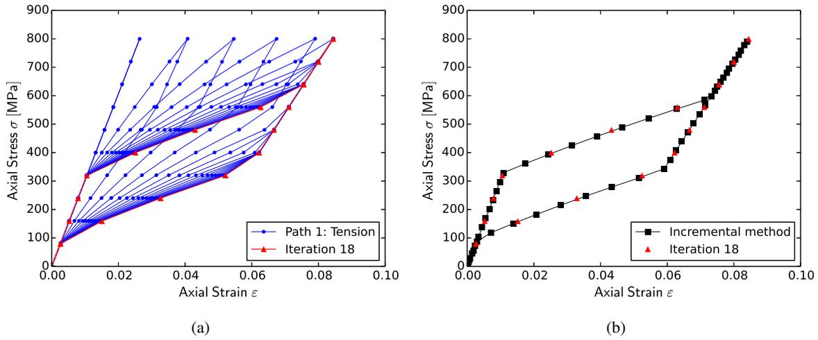
FIGURE 3 – Simulated stress-strain behavior for the case of uniaxial tension.
