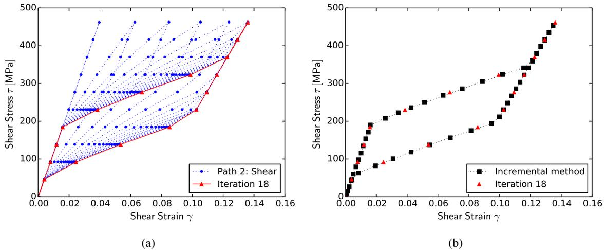
FIGURE 4 – Simulated stress-strain behavior for the case of pure shear.
