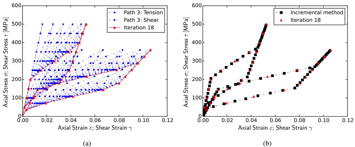
FIGURE 5 – Simulated stress-strain behavior in tension and in shear for the case of combined loading.
