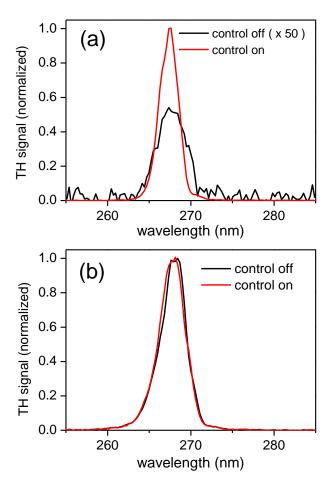
Fig. 5. Effect of crossing filament on the TH generation. The focal lens for (a) and (b) are 1000 mm and 200 mm respectively. The focal length for the control pulse was 500 mm and the control pulse energy was 380  $\mu$ J, similar to that in ref [24].
