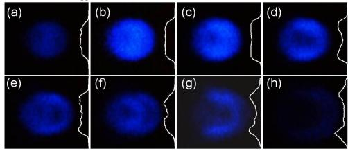
Fig. 4. Far field profile of the third harmonic radiation for different air pressures. The focal length is 1000 mm and the paper screen is 75 cm away from the geometrical focus. The incident pulse energy is 1.2 mJ. From (a) to (h), the pressures are 30, 70, 200, 300, 350, 430, 600, 1000 mbar, respectively.
