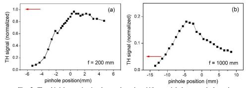
Fig. 2. The third harmonic signal pass through a 110  $\mu$ m pinhole scanned along the filament. (a) f = 200 mm. (b) f = 1000 mm. The origin (z = 0 mm) is defined as the geometrical focus in each cases.
