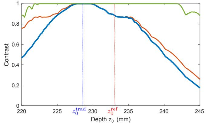
**Fig. 5.** Contrast curves versus depth: with defocus and magnification only (green), with diffraction and magnification only (orange) and with the three effects combined (blue). Depths  $z_0^{\text{ref}} = 233$ mm and  $z_0^{\text{trad}} = 228.6$ mm. Note that the small oscillations are due to pixel discretization of the signal.
