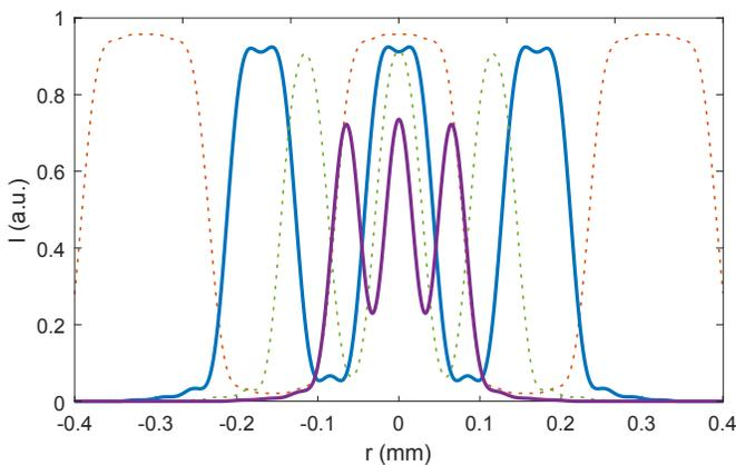
**Fig. 4.** Simulated 1D raw image with the three effects versus position  $r$  on the detector for different depths  $z_0$ :  $z_0^{\text{ref}} = 233$ mm (blue), 231mm (dotted orange), 235mm (dotted green), and 240mm (purple, same depth as in Fig. 3).
