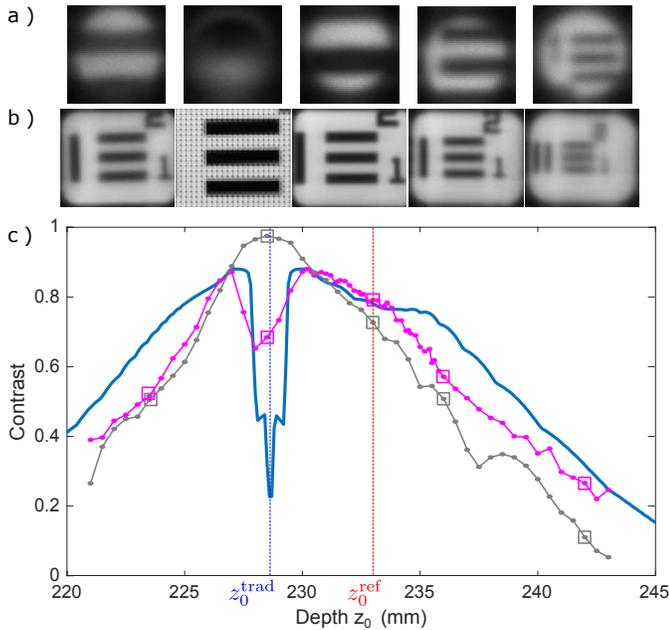
**Fig. 6.** a) Raw sub-images acquired at planes:  $z_0 = 223.5, 228.5, 233, 236, 242$ mm; b) Corresponding reconstructed images; c) Comparison of the simulated contrast curve (blue) and experimental contrast curve measured on raw sub-images (pink) and on reconstructed images (gray). The gap located around  $z_0^{\text{trad}} = 228.6$ mm is due to the large magnification that makes the bars exceeding the sub-image size.
