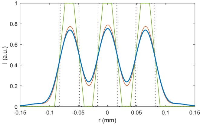
**Fig. 3.** Simulated 1D raw image of the test object versus position  $r$  on the detector with the effect of defocus only (green; contrast = 1), with diffraction only (red; contrast = 0.59) and with both effects combined (blue; contrast = 0.52), calculated at a depth  $z_0 = 240$ mm, compared to the image with no effect (dotted black; contrast = 1).
