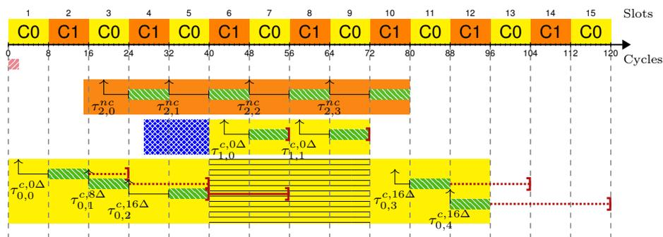
■ **Figure 6** Memory blocking delays considering criticality inheritance (SHDi).
