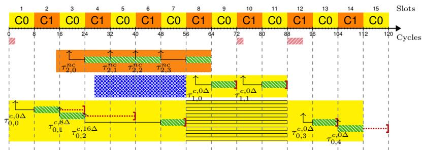
■ **Figure 3** Impact of slack accumulation on the memory blocking time for TDMs.
