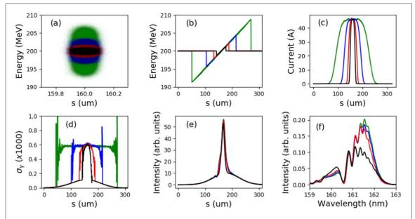
**Figure 4.** Influence of the initial energy spread on the FEL spectrum. Longitudinal energy distribution (a) at the LPA source and (b)–(c) at the undulator entrance, (c) longitudinal energy spread and current at the undulator entrance, FEL temporal profile (e) and on-axis spectrum (f) at the undulator exit. The initial energy spread is varied from  $\pm 2\%$  (green),  $\pm 1\%$  (blue),  $\pm 0.5\%$  (red) and  $\pm 0.3\%$  (black). Other parameters from table 1.
