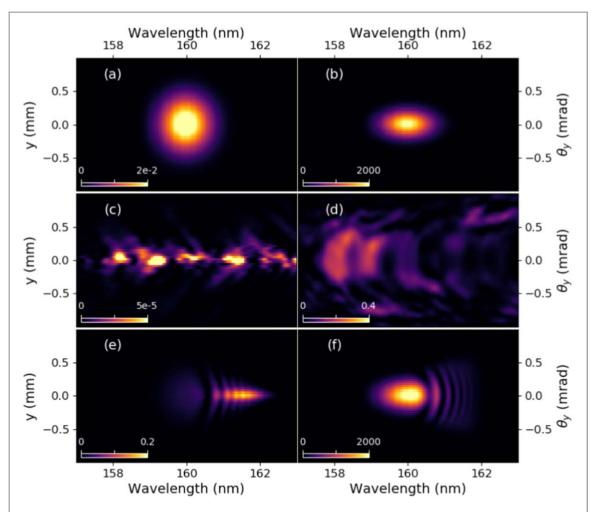
**Figure 2.** Simulated spatio-spectral distribution of the radiation at the undulator exit in the near- (left) and far-field (right). (a) and (b) Seed only ( $P_{\text{seed}} = 10 \text{ kW}, Q = 0 \text{ pC}$ ), (c) and (d) Spontaneous emission only ( $P_{\text{seed}} = 0 \text{ W}, Q = 20 \text{ pC}$ ) and (e), (f) FEL case ( $P_{\text{seed}} = 10 \text{ kW}, Q = 20 \text{ pC}$ ). Other parameters from table 1.
