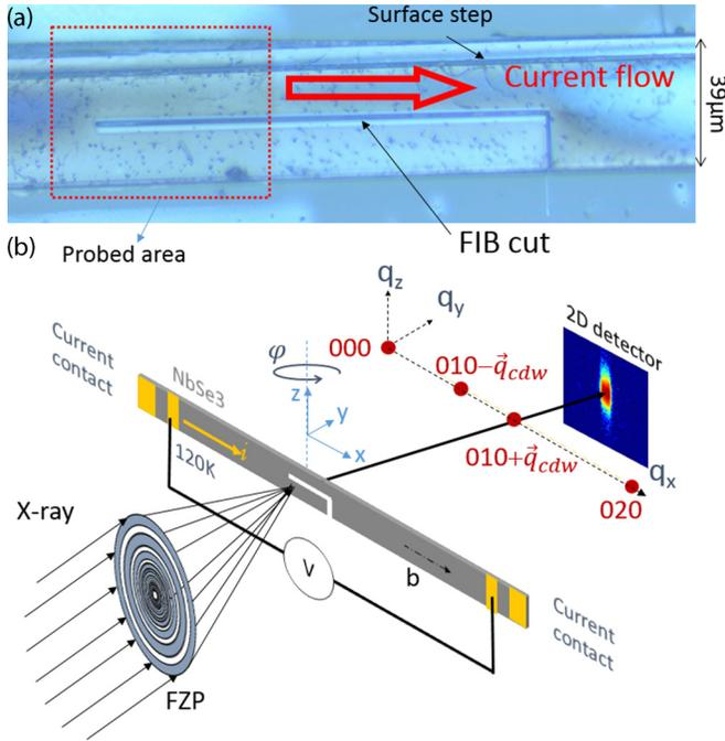
FIG. 1. (a) Optical image of the NbSe<sub>3</sub> sample showing the line cut made by the FIB, the presence of one step on the surface, and the area probed by the focused x-ray beam with 1  $\mu\text{m}$  steps. (b) Schematic drawing of the experimental setup. The sample frame is rotated with respect to the laboratory frame by an angle  $\varphi$ . The CDW is along the  $q_x$  direction, which corresponds to the  $\vec{b}$  axis of NbSe<sub>3</sub>.
