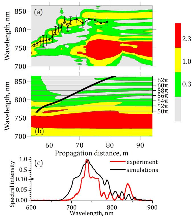
**Fig. 3.** Resolved over the distance  $z$  spectra of the Stokes side of the supercontinuum in the experiment (a) and simulations (b) and their slice at 90 m (c). Black circles in (a) repeat the measured dependence of *averaged*  $\lambda_{Stokes}(z)$  from Fig. 2(c); it differs slightly from the color map as the latter is based on *single-shot* spectra. Black curve (right axis) in (b) shows the simulated dependence of  $B$ -integral on  $z$ .
