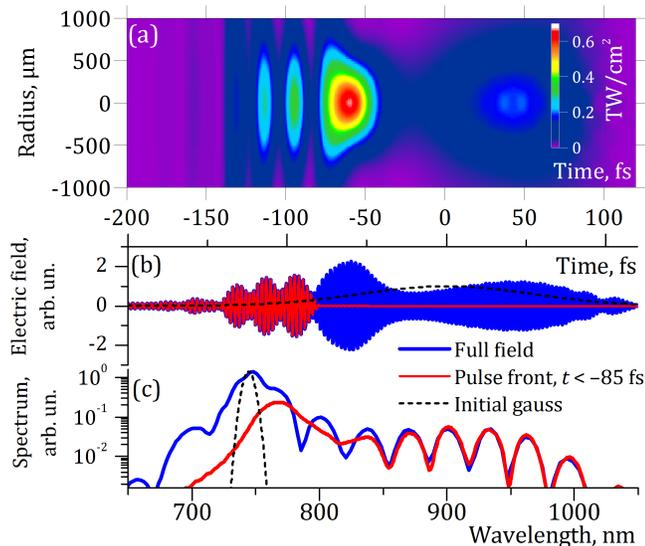
**Fig. 4.** Simulated (a) spatio-temporal distribution of the pulse intensity, (b) on-axis light field and (c) integrated over beam spectrum of the whole pulse (blue curve) and of the pulse train in its front ( $t < -85$  fs, red curve) at  $z = 80$  m.
