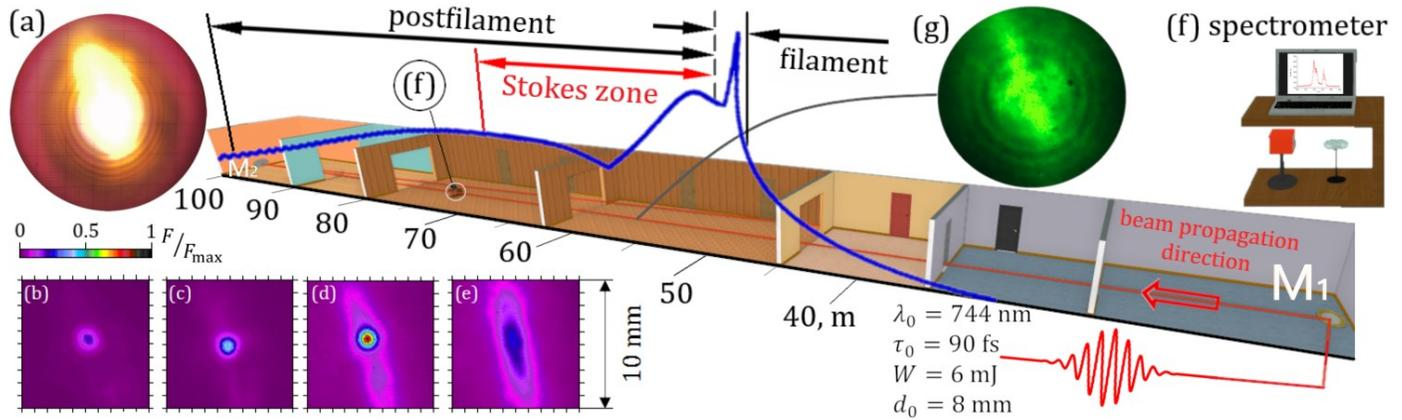
**Fig. 1.** Sketch of the experiment in the corridor with the trolley (f) equipped with spectrometer and CCD camera. Blue curve is variation of the simulated peak intensity vs. propagation distance from the compressor output. (a) Conical emission on the far wall of the corridor. Measured transverse fluence distributions at (b) 100 m, (c) 80 m, (d) 50 m, (e) 40 m. (g) Transverse beam profile observed at 56 m using low-pass spectral filters to increase the contrast of rings.
