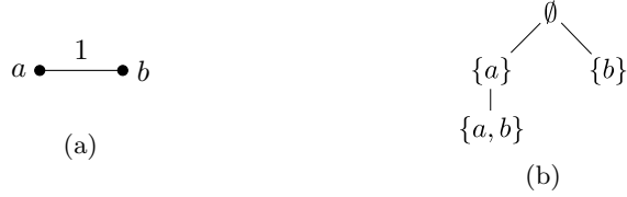
Figure 5: (a) A graph and (b) its corresponding enumeration tree obtained with Algorithm A_1 .
