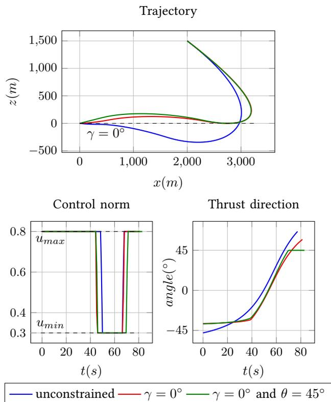
FIG. 3 – Simulation results for  $q = 0$  without glide-slope or pointing constraint (blue), with only a glide-slope constraint of  $\gamma = 0^\circ$  (red) and with glide-slope and pointing constraints for  $\theta = 45^\circ$  (green).
