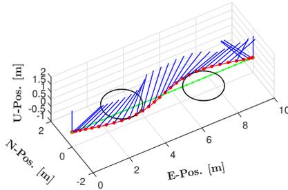
**Figure 1: A perspective view of the problem setup. The obstacles are represented by the black circles. The red dots and blue lines represent the time discretized positions and thrust vectors, respectively. The green dots represent the initial trajectory (i.e., a straight line). The motion of the vehicle is from left to right.**
