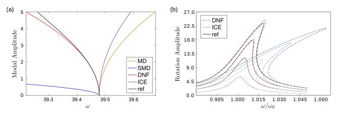
Figure 1: (a) Backbone curves for a linear beam resting on a nonlinear elastic foundation, comparison between QM methods with either full modal derivatives (MD) or static modal derivatives (SMD), Implicit condensation (ICE), and direct normal form (DNF). Reference solution in black. (b) Comparison between Implicit condensation (IC), direct normal form (DNF) and full-order solution for a MEMS micromirror.
