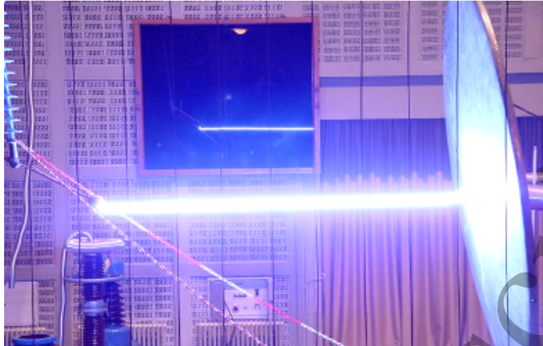
Figure 7: Picture of a laser-guided negative discharge. Adapted with permission from [Rodriguez2002]. © Optical Society of America
