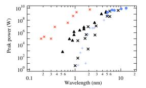
Figure 3: Short wavelength spectral range covered by the HHG seeded FEL sources. Seed 30-50 kW, 50 fs-FWHM: LEL1 (Phase 2), (+) planar (o) helical configuration ; LEL2 (x) E=1 GeV, ( $\Delta$ ) E=1.2 GeV; \* LEL4 in Phase 3.
