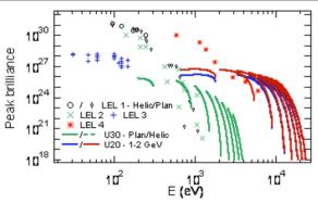
Fig. 4 : Peak Brilliance of ARC-EN-CIEL (10 kHz assumed for phase 2, 20 mA average current for phase 3).
